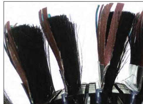
Composition with thrust filament, abrasive and empty space. Proposal suitable for the brushing and profiled sections where it is necessary to go deep (window, flat complex profiles). Loading pressure from 15 to 40 mm.
