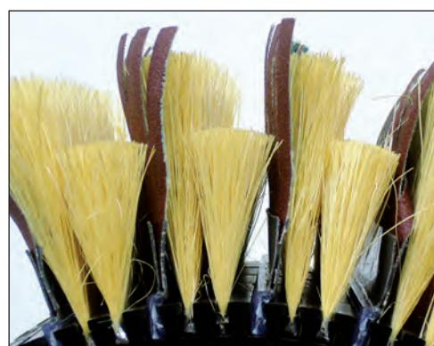
Composition with double thrust filament and abrasive. Proposal suitable for the brushing of profiled sections, where considerable pressure is needed (gleaning, radius, homogeneity on joint area between panels). Loading pressure from 5 to 25 mm.
